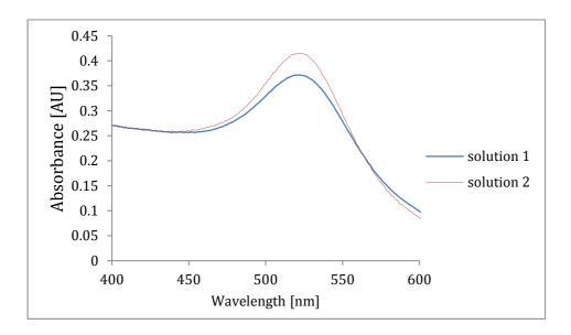
For solution **1** the maximum of absorbance is 0.37 at 522 nm and for solution **2** the maximum is 0.41 at 522 nm.
